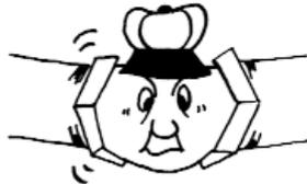
**Proper support** will prevent strain and distortion due to sagging pipe. Hangers and supports should be close enough and properly aligned.
