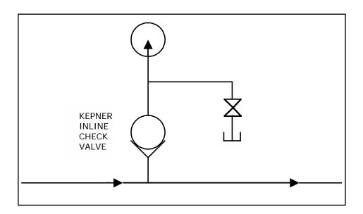
The simple circuit shown above is an integrator for use in cases of repetitive shock or single surges of duration within the response rate of the gage. On each successive pressure rise an increment of fluid is trapped in the gage line until the gage line pressure balances the surge pressure. When the gage reading stabilizes, the reading will be very close to the peak surge pressure.
