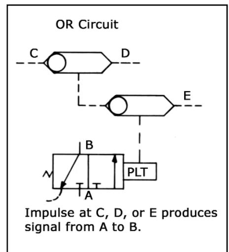
Impulse at C, D, or E produces signal from A to B.
